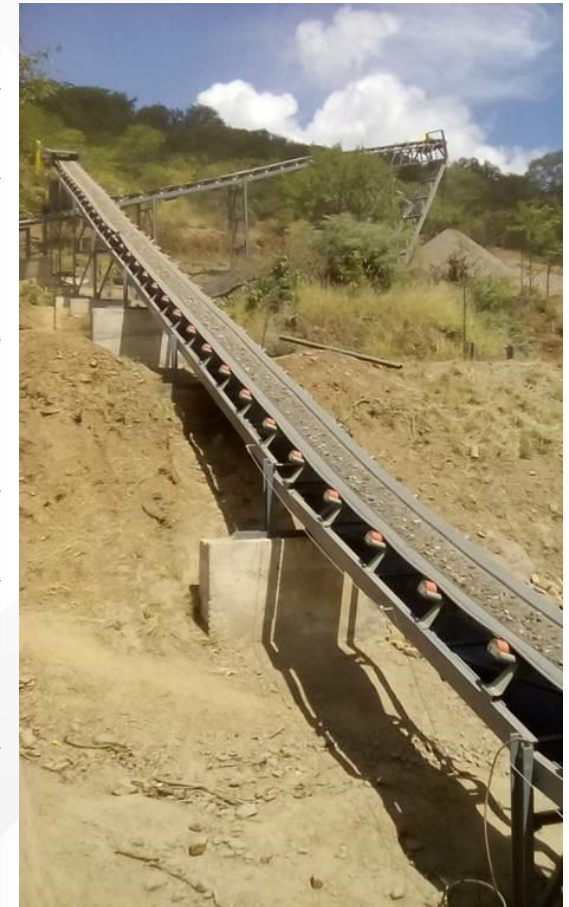
Conveyor Belts from XRT Sorter
